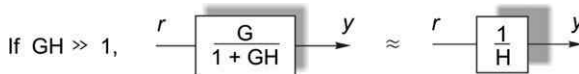
Figure A1.5 Simplification of closed-loop system model when loop gain ( GH ) is much greater than 1.
