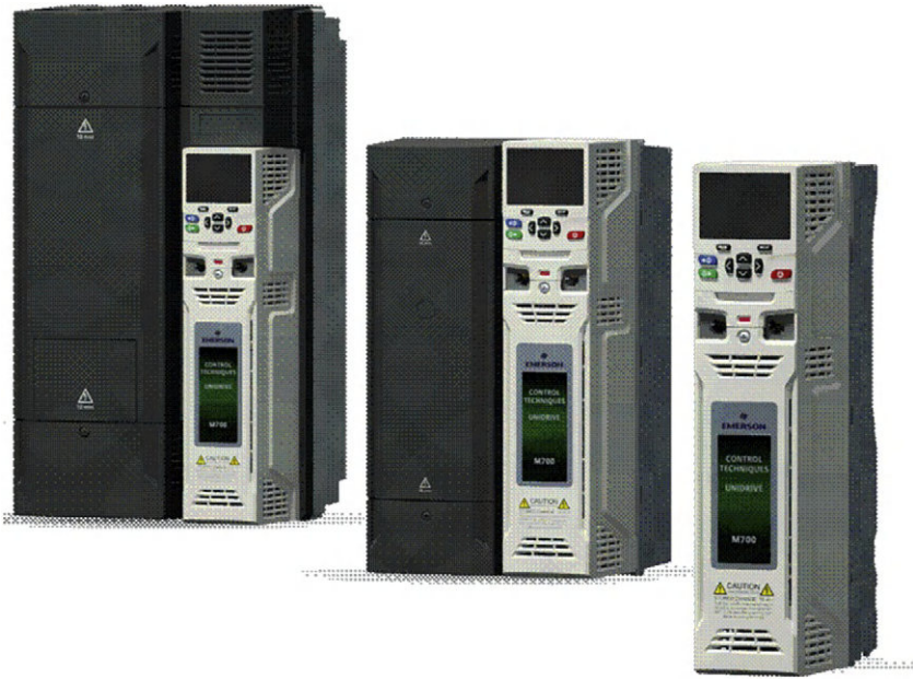
Plate 2.1 Emerson – Control Techniques Unidrive M700 industrial a.c. drives. These three are from the lower end of the range of seven that extends to 315 kW. The right hand unit is 4 kW/5 HP (380 mm high), while the left hand unit is 45 kW/60 HP. (Courtesy of Emerson – Control Techniques)
