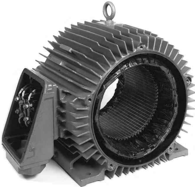
Plate 5.1 Stator of three-phase induction motor. The semi-closed slots of the stator core obscure the active sides of the stator coils, but the ends of the coils are just visible beneath the binding tape. (Courtesy of Brook Crompton)
