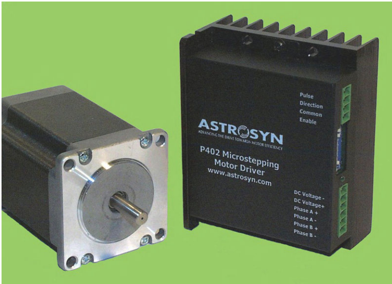
Plate 10.3 This bipolar chopper mini-stepping drive with integral heatsink provides a range of step divisions up to 25,600 steps/rev and allows drive current to be set from 0.25 A to 2.0 A with supply voltage from 14 V to 40 V. (Courtesy of Astrosyn)
